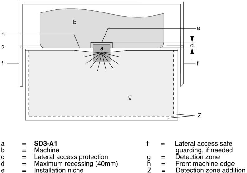
**Fig. 5.4-2:** Recessed installation within the machine contour
