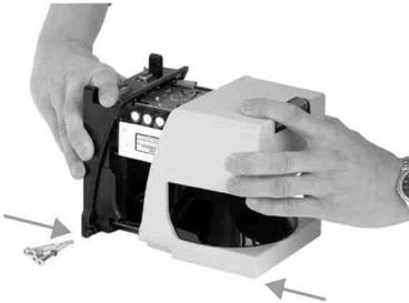
After that, carefully screw in the screws on the rear wall of the housing, working back and forth around the circle from screw to screw.
