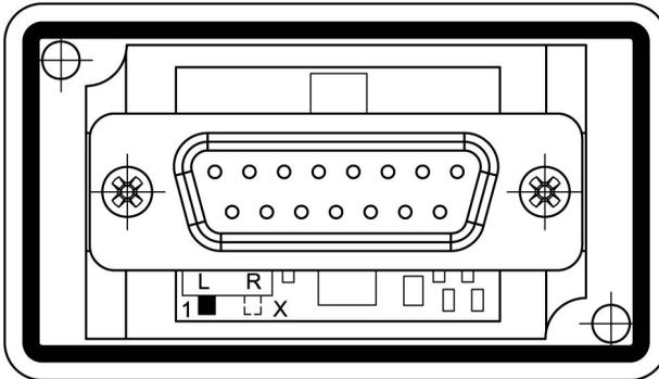
Fig. 10.5-1: SD3-A1 ConfigPlug with switch setting "1"
