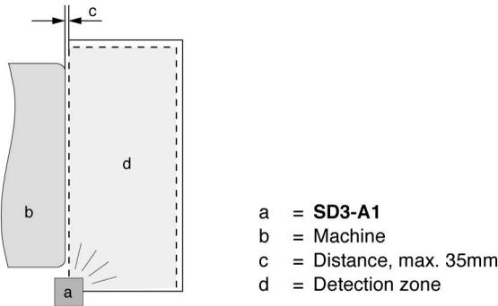
Fig. 5.4-3: Lateral external scanner mounting without an undercut
