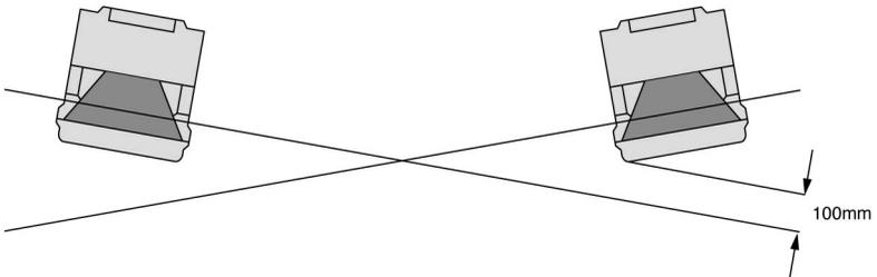
**Fig. 5.2-3:** Installation without height offset (crossed alignment)
