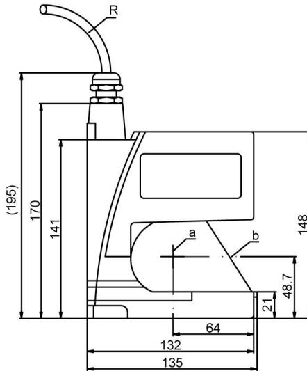
R = Smallest bending radius = 50mm
