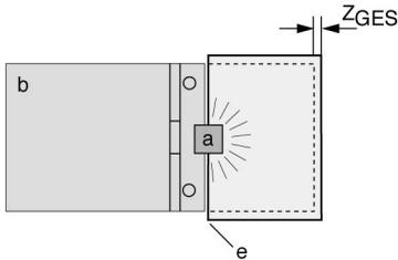
**SD3-A1 recessed into the front of a vehicle**
