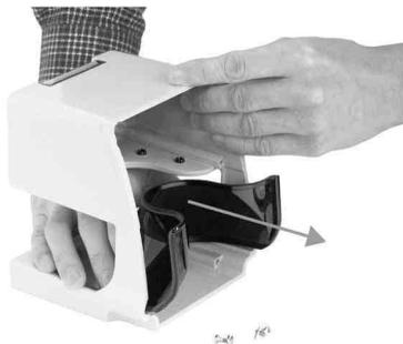
Press the old optical window out through the rear (through the housing)
