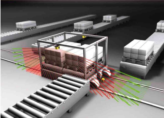
**Fig. 4.6-1:** Bild 6.3-1 guarding the sides on AGVs
