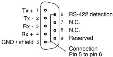
**Fig. 1.9-1:** Interface pin assignments with a view to the **SD3-A1**
