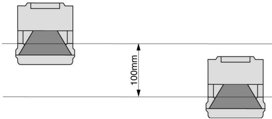
**Fig. 5.2-2:** Installation with height offset (parallel alignment)
