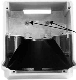
When assembling the housing, note that the two retaining bolts slide into the rubber sleeves provided for them. To do this, carefully join the two housing parts on a level surface.
