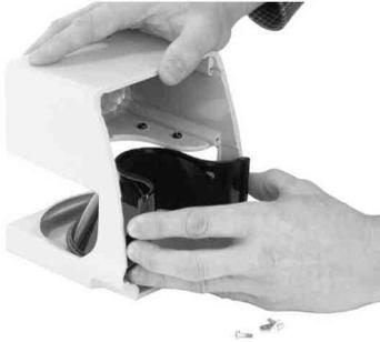
Hold the new optical window by the sides and carefully insert it in the correct position, pressing the optical window together slightly as you do so. Make certain the rubber seal is not damaged. Make certain it is in the groove in the housing designed for that purpose.
