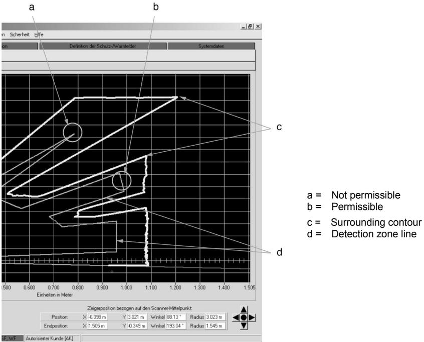
The maximum selectable detection zone radii vary depending on the type of contour:
