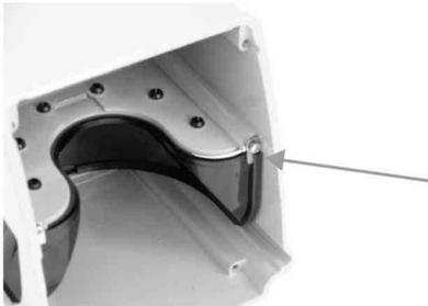
Check to make sure the optical window is seated correctly. There should be no gap between the optical window and the housing that lets light through.
