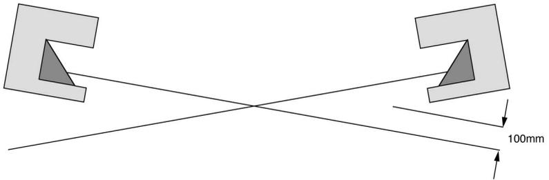
**Fig. 5.2-4:** Opposing installation without height offset (crossed alignment)
