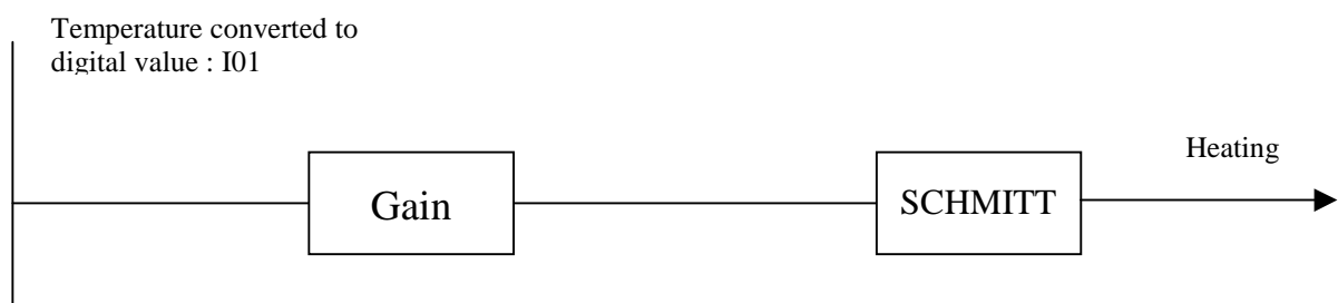
Fig. 1.55 Logic diagram for temperature control.
