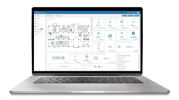
The Dashboard is a user-friendly interface where admins can monitor and interact with connected devices though graphs, charts and other tools. It allows users to manage every aspect of their connected devices as well as gain insight on the environment through visualization of device data.
