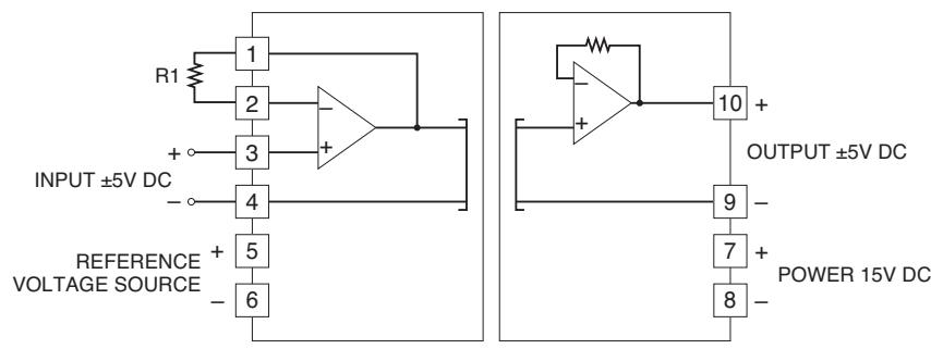
■ Inverting amplifier circuit: Basic example of  $G = -1$  (output inverted to the input)
