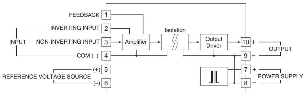
Note. The reference voltage source is common to the COM (-), terminal 4.
