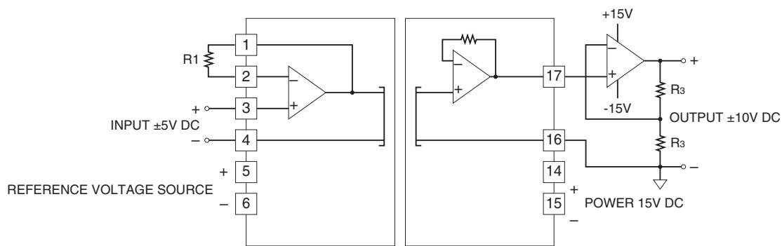
Non-inverting circuit  $G = 1 + R_3 / R_2 = 2$
