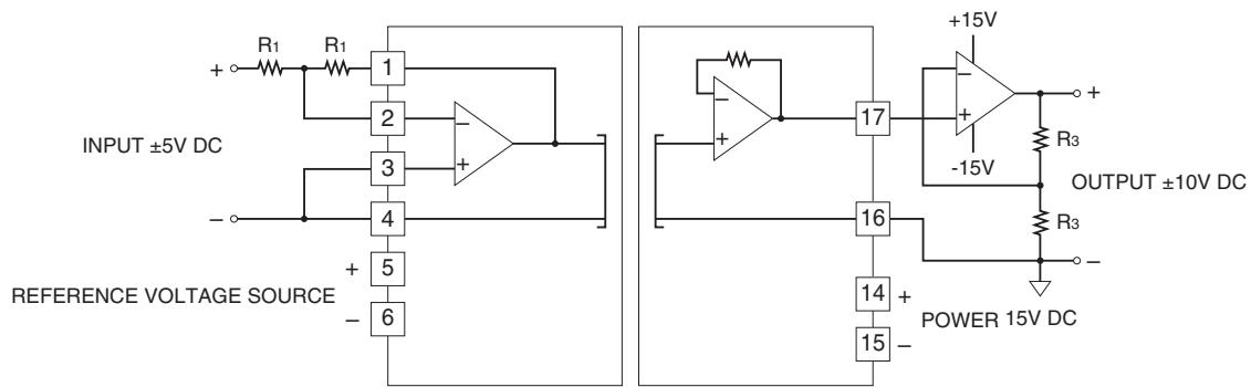
Inverting circuit  $G = -(1 + R_3 / R_2) = -2$
