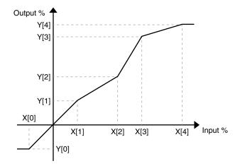
If a value equal to the input % value is not set in X[n], extract the closest value in each of the positive and negative directions from the set X[n], and then linearly complete the two points as shown in the formula below to obtain the output % value.
