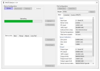
The upload will be completed in a few seconds, and the loaded parameters will be displayed in the file settings on the right side of the screen and can be edited.
