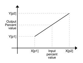
If the input value in percent is out of the table, set Y[n] that pairs to the closest X[n] as output value in percent.
