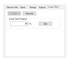
Enter the output value in percent into the field and click set to change the output of the device to the entered output value in percent.
