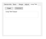
Click Fixed to fix the output at the current status, so that the output will not follow any change in the input. The screen will change into following and output can be controlled.
