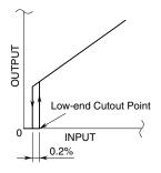
When the output low limit is set to a value higher than 0%, the input below the low-end cutout point is forced to the value, not 0%.
