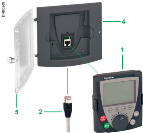
Using the remote graphic display terminal on enclosure door: 1 + 2 + 4 (+ 5, if IP 65)
