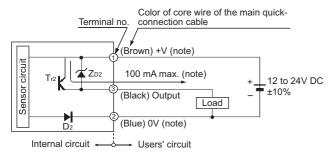
50mA max. if five or more connector type FX-301(P) amplifiers are connected in cascade.
