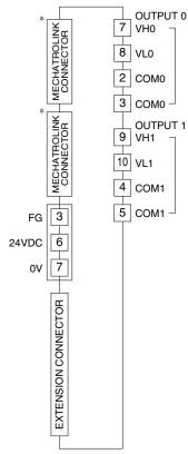
\*MECHATROLINK connectors are internally connected. The network cable can be connected to either one.
