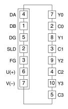
Caution: FG terminal is NOT a protective conductor terminal.
