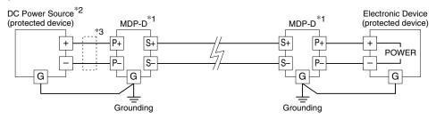
The MDP-D is not applicable to protect two-wire transmitters. To protect two-wire transmitters model MDP-24-1 designed to yield only small leakage current is suitable.
