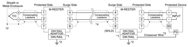
\*1. Oxide film on the surface of an aluminium rail may lower the electric conductivity between this module and the ground. Use a steel or copper rail.
