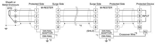
\*1. Oxide film on the surface of an aluminium rail may lower the electric conductivity between this module and the ground. Use a steel or copper rail.
