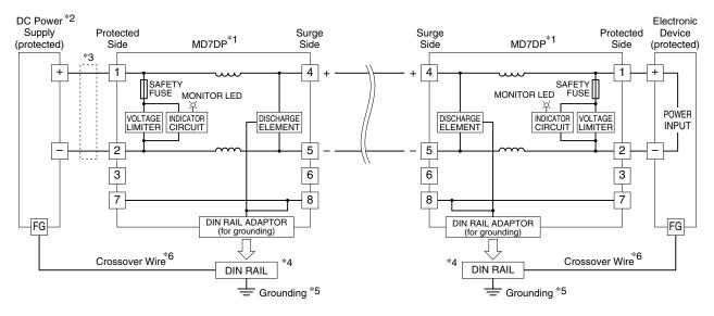
\*1. The MD7DP is not applicable to protect two-wire transmitters. To protect two-wire transmitters, model MD7ST designed to yield only small leakage current is suitable.
