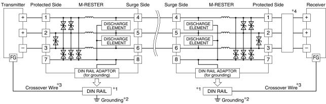
\*1. Oxide film on the surface of an aluminium rail may lower the electric conductivity between this module and the ground. Use a steel or copper rail.
