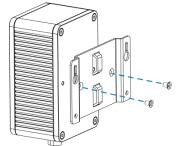
2. Drill 4 holes on the wall according to the bracket, then fix the wall plugs into the wall.
