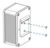
2. Hang the device to the DIN rail. The width of DIN rail is 3.5cm.
