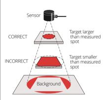
We normally recommend that the target should be at least twice the size of the measured spot for maximum accuracy.
