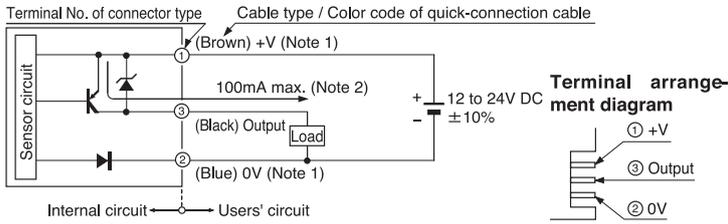
Notes: 1) The quick-connection sub cable does not have +V (brown) and 0V (blue). The power is supplied from the connector of the main cable.
