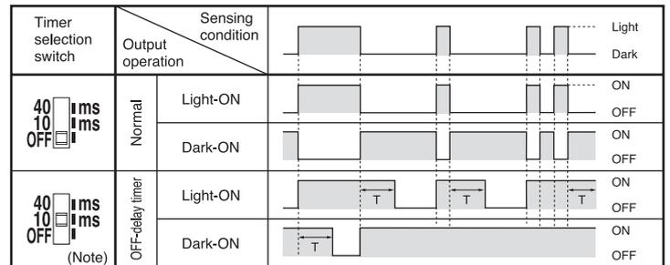
Note: The diagram shows the case when 10ms delay time is selected.
