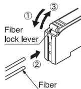
Notes: 1) In case the fiber cables are not inserted to a position where they stop, the sensing range reduces. In case of a flexible fiber, take care that it may bend inside the amplifier, during insertion.
