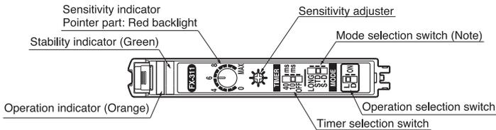
Note: The mode selected by the mode selection switch for FX-311B(P) and FX-311G(P) is 'LONG', 'STD' or 'FAST'.
