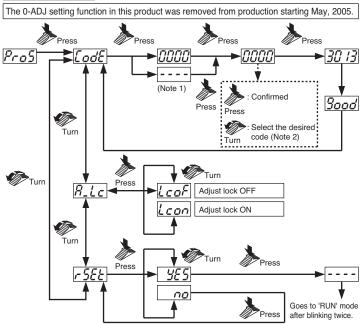
Notes: 1) When any code other than the codes given in the Code setting table below is used, ' - ' is displayed. The factory setting is "DDV '. 2) When the code setting function is used, refer to the 'Code setting table' given below.
