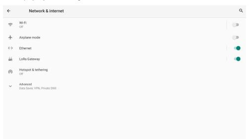
Select Ethernet IP mode as **static** or **dhcp** and plug the Ethernet cable to Ethernet port of device to access the network.
