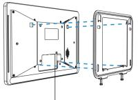
4. Fix the IoT Display to the bracket by tightening the 2 screws at the bottom of the bracket.
