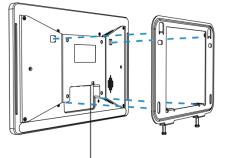
6. Fix the IoT Display to the bracket by tightening the 2 screws at the bottom of the bracket.
