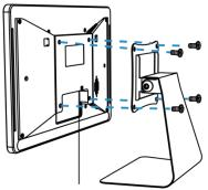
2. Fix the IoT Display to the VESA desktop stand by tightening the screws.
