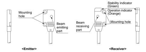
Thru-beam side sensing type: EX-11E , EX-13E , EX-19E **EX-11SE** , **EX-13SE** ,
