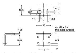
(Note):The sensor bracket is an object for satandard-beam type. It cannot be used for narrow-beam type.
