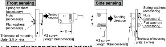
In case of using mounting bracket (optional) The sensor bracket is an object for satandard-beam type. It cannot be used for narrowbeam type.
