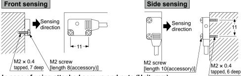
In case of using attached screws and nuts (Unit: mm)
