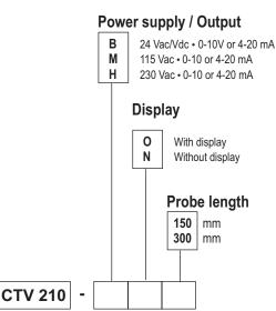
$\textbf{Example: CTV210-MN150} = \text{air velocity and airflow transmitter type CTV 210}, with 115 \,\text{Vac power supply, without display, with hotwire probe length 150mm}.$
