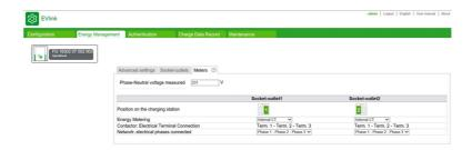
Energy metering is achieved per charge point for the charging stations with two charge points. This can be done without adding meters when it is based on the measurement of the charging current using current transformers inside the charging station, and on the value of the measured phase neutral voltage that has been entered in the **Phase-Neutral Voltage measured**.
