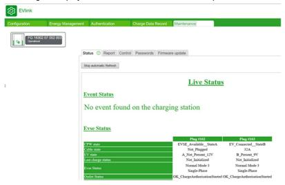
Cable State is the current capability of the cable connected to the charging point (maximum ampere value). The following table describes all possible values:
