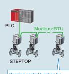
Opening control function by analog signal is also standard Operation Signal (4-20mA DC) Opening Signal (4-20mA DC)
