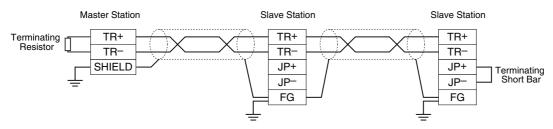
Note: Be sure to use the terminator(s) located at both ends of the modules.
