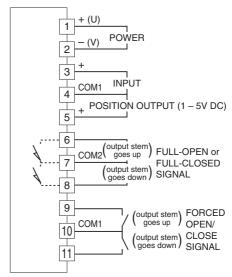
Full-open/-closed signals and forced open/close signals are optional.
