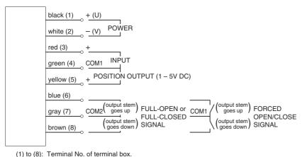
• With Both Full-open/closed Signal and Forced Open/Close Signal
