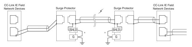
\* LAN cable's shield wire (SHLD) is 'earthed' when shortcircuit bar is connected. Make sure to connect the shortcircuit bar when you use shielded LAN cable.
