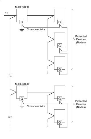
\*1. Fieldbus devices complying with IEC 61158-2 operate by a supply voltage between 9V and 32V DC.
