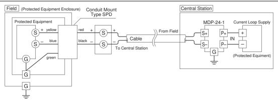
Connect the Conduit Mount Type SPD's green leadwire to the ground terminal inside the protected equipment enclosure to ground through the enclosure's outside ground terminal.
