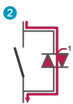
Start: conduction through the semiconductor.
