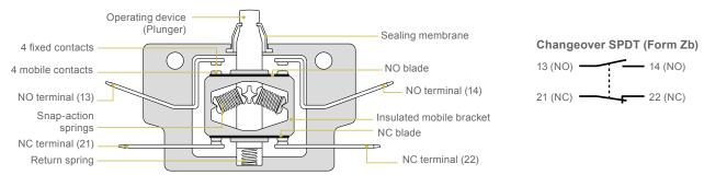
NO and NC circuits are electrically separated, and can be used at opposite polarities.
