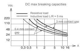
DC breaking capacity can be significantly increased by using different means, if necessary in combination:
