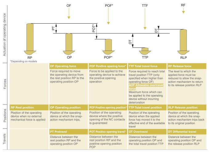
The reference point for the figures given for travels and forces is a point F located on the top of the plunger in the case of a plain microswitch, or, generally, 3 mm in from the end of a flat lever. The reference point for the positions is one of the fixing holes, unless otherwise indicated.
