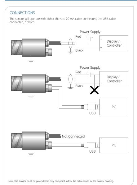
PyroUSB Series infrared pyrometers measure temperatures from -40°C to 2000°C accurately and consistently, with an outstanding response time of 200 ms. The 4 to 20 mA output is compatible with almost any indicator, controller, recorder or data logger. without the need for special interfacing or signal conditioning.
