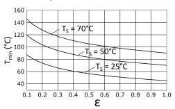
Graph showing the minimum measurable object temperature (Tmin), determined by surface emissivity (ε) and sensor temperature (TS).
