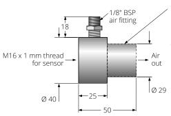
Removable spigot fitted to type APSN for use with -151, -301 and -CF models. Not fitted to type APSW for -21 models.
