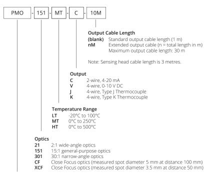
РМО PyroMini OEM infrared temperature sensor with miniature sensing head and separate electronics module
