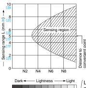
The sensing region (typical) is represented by oblique lines in the left figure. However, the sensitivity should be set with enough margin because of slight variation in products.
