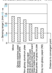
The bars in the graph indicate the sensing range (typical) for the respective material. However, there is a slight variation in the sensing range depending on the product. Further, if there is a reflective object (conveyer, etc.) in the background of
