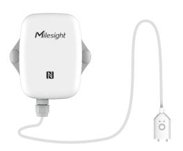
EM300-SLD is a compact spot leakage detection sensor for detecting presence of water (or other liquids) and transmitting alarm using LoRaWAN<sup>®</sup> technology. With this low power consumption technology, EM300-SLD can work up to 5 years with 4000 mAh battery. Combining with Milesight LoRaWAN<sup>®</sup> gateway and Milesight IoT Cloud solution, users can manage all sensor data remotely and visually and receive alarms via mobile APP.
