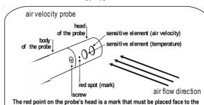
airflow. Then, the probe is perpendicular to the airflow.
