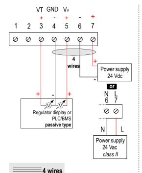
To make a 3-wire connection, before powering up the transmitter, please connect the output ground to the input ground. See drawing below.
