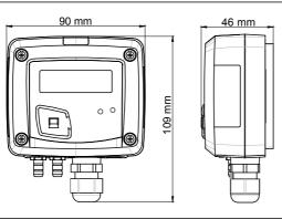
Material: ABS V0 as per UL94 Protection: IP65 Display: LCD 10 digits. Size: 50 x 17 mm Height of digits: Value: 10 mm; Unit: 5 mm Connections: safety Ø6.2 mm Cable gland: for cables Ø8 mm maximum Weight: 143 g
