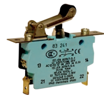
Mixed connections: NO screw with clamp / NC quick-connect 6.3 x 0.8, 90° downward folding
