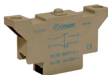
Economic version (839930): SPDT form Za without positive opening, Ø 3.2 mounting holes on top face, screw terminals
