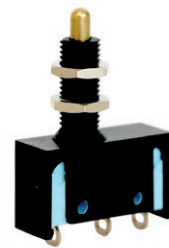
Telescopic plunger with 3 mm overtravel and with M6 x 0.75 threaded barrel
