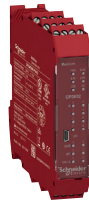
Minimum size of hardware: a safety controller CPU used as standalone: 8 safety digital inputs + 2 OSSD pairs or 4 single channel OSSD + 2 or 4 status outputs
