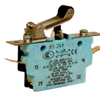
Mixed connections: NO quick-connect 6.3 x 0.8 / NC screw with clamp
