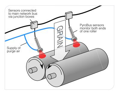
Two PyroBus sensors (model PB21) are aimed at the milling surface of one roller in each machine. Monitoring both ends of the roller helps ensure a hazardous temperature at only one end is properly caught.
